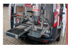
Mobile fire extinguisher service unit MFS ready for operation in van.
