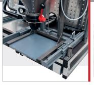
Lowerable set-up table for the filling of fire extinguishers.
