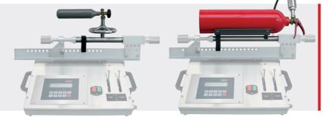
• Art. No. 186103 Filling head F2 for exterior CO<sub>2</sub> cylinders with turning valve up to 300 g.
